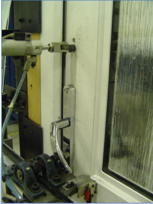
Key rotates to unlock, handle lowers to disengage.
