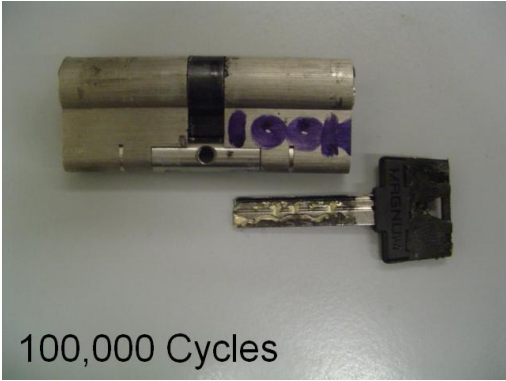
Cylinder after 100,000 Cycles
