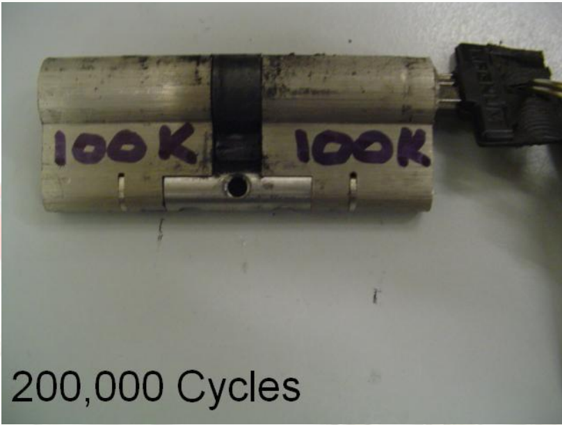
Cylinder after 200,000 Cycles
