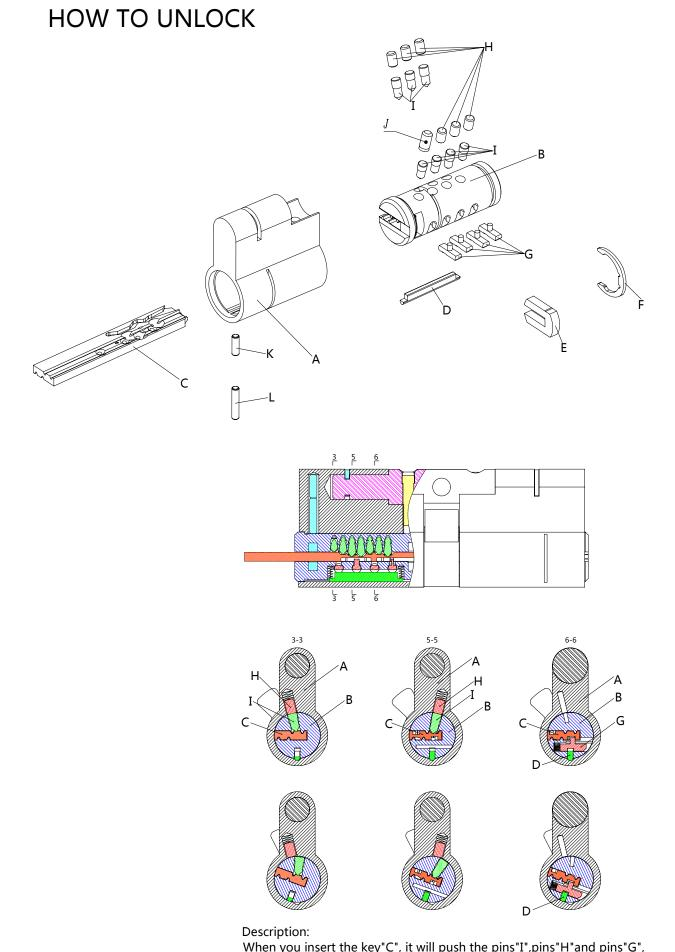
When you insert the key"C", it will push the pins"I",pins"H"and pins"G", the teeth on the key"C" will make all the pins move to the right place where like the images showed. After you insert the key, the pin"H" can't make the cylinder"B" get stuck anymore, and the pins"G" will move to the right position to let the gap on it suit the position of part"D". So the cylinder"B" can be turned in the lockbody"A".
